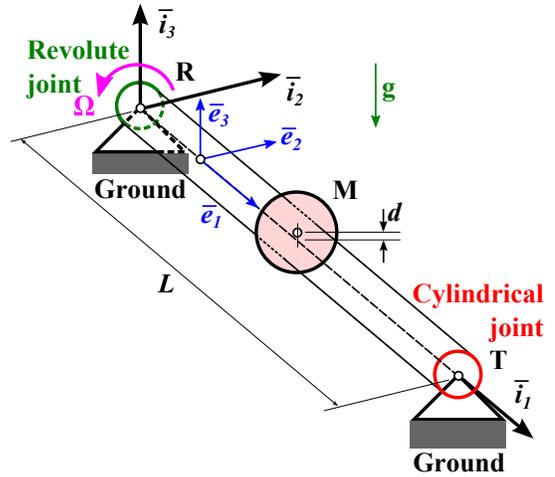
Figure 1: Configuration of the rotating shaft
