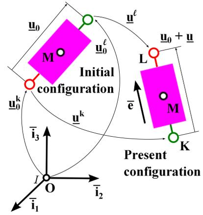
Figure 2: Configuration of the force element interface.
