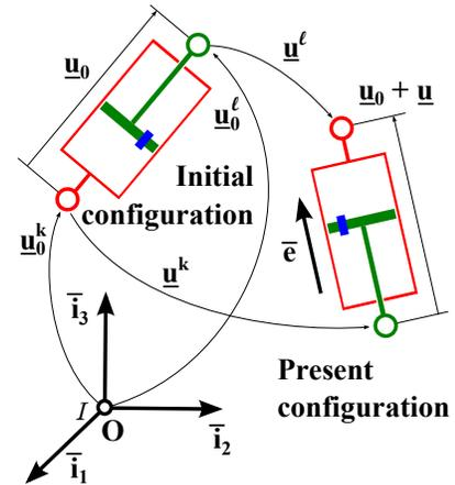
Figure 1: Configuration of the force element interface.
