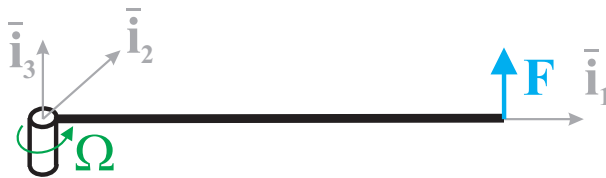
Figure 8: Rotating cantilevered beam subjected to transverse tip force.
