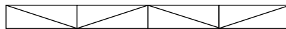
Fig. 13b. Two elements in width mesh, the warping feature is not shown, for clarity.
